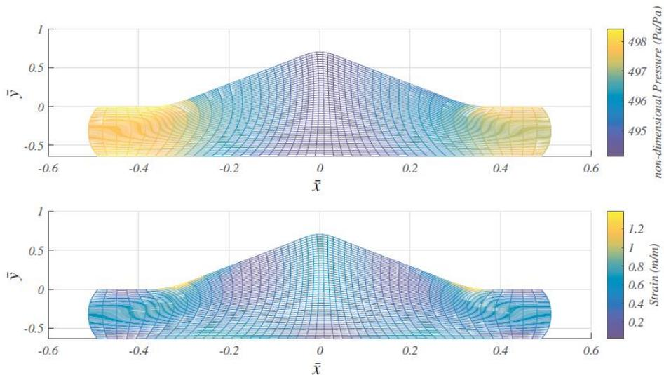
**Figure 3.** Non-dimensional pressure and strain for one feature at the end of mold filling process.
