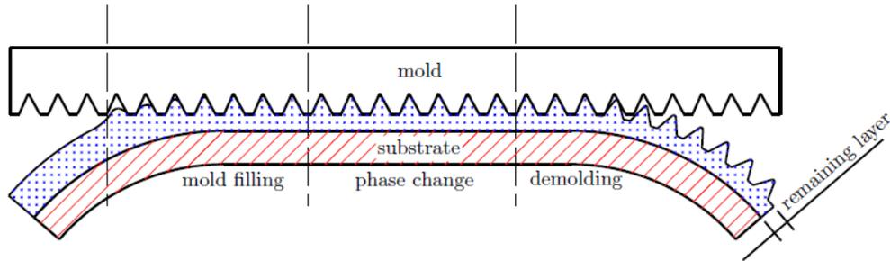
**Figure 1.** Mechanical sub-processes of R2RNIL process.
