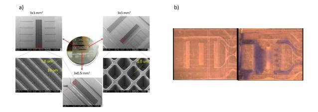
**Figure 1:** SEM images (Figure a) of the final pattern realise for the microfluidic chip (showed in the middle). Figure 1b shows the microfluidic chip before and after being filled with whole blood.
